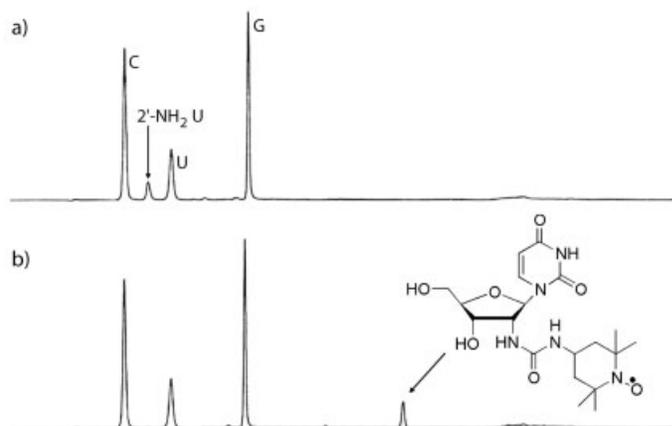
**Fig. 8.5.** HPLC analysis of enzymatically digested RNA (a) enzymatic digestion of 5'-GCU C(2'-NH<sub>2</sub> U)C UGG CCC; (b) enzymatic digestion of the product of the 2'-NH<sub>2</sub>-modified oligonucleotide from a after reaction with isocyanate 4. HPLC chromatograms were obtained as in Fig. 8.4.
