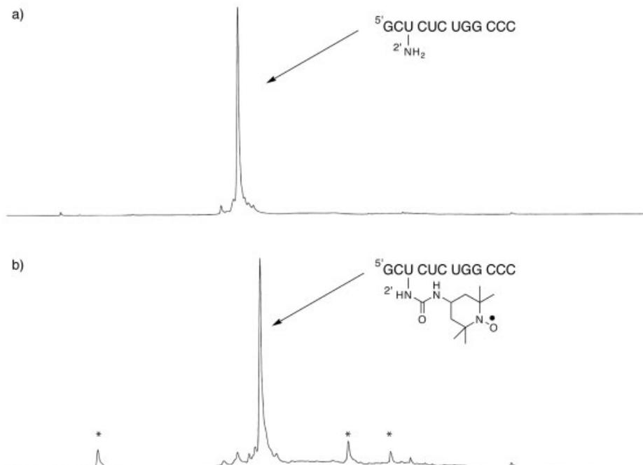
**Fig. 8.4.** HPLC analysis of 5'-GC(2'-NH<sub>2</sub> U) CUC UGG CCC before (a) and after (b) reaction with **4** which shows 95% conversion to the labeled RNA of later retention time. The asterisks correspond to **4** and its hydrolysis products. HPLC chromatograms were obtained at 260 nm using an analytical column (C18, 4.6 × 250 mm, 5-μm column) run at 1.5 ml/
